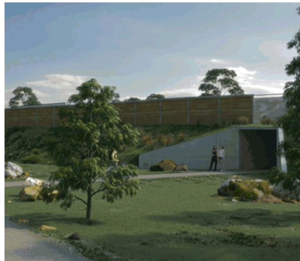
Proposed pedestrian underpass at Braeside Park - ground level (source: https://roadprojects.vic.gov.au/projects/mordialloc-freeway/view-the-ees ). Sheer wing-walls create a harsh entry appearance and palette for graffiti.
