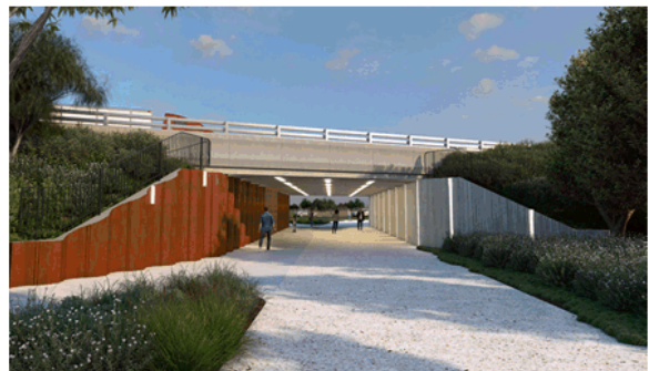
Drysdale Bypass splayed wing walls with integration of planting and cladding to create an attractive and welcoming environment.
